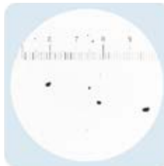
NAS 7 ISO 18/15/13 Typically new oil as delivered in new certified mini containers
