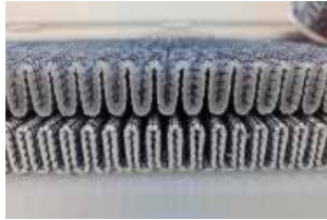
The Filter Media has absorbed water
